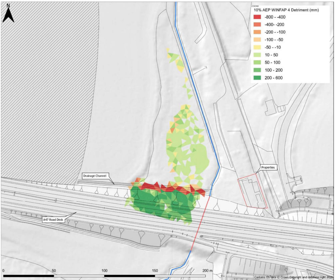
Figure 6-1: 1 in 10-year detriment flood map. Contains OS data (Crown copyright and database rights 2020).
