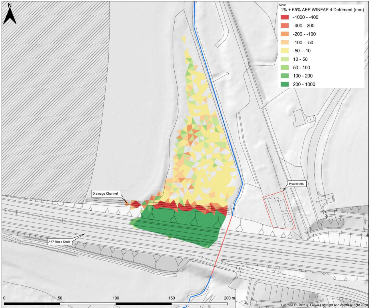
Caption 7-9 - The 1 in 100-year plus 65% climate change allowance flood depth difference map
