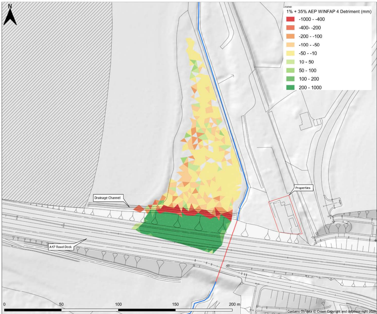
Caption 7-8 - The 1 in 100-year plus 35% climate change allowance flood depth difference map
